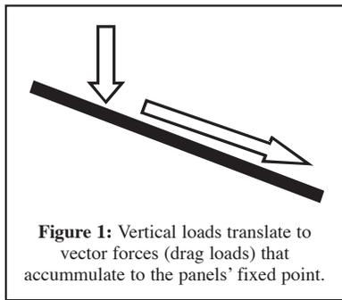
**Figure 1:** Vertical loads translate to vector forces (drag loads) that accumulate to the panels’ fixed point.
